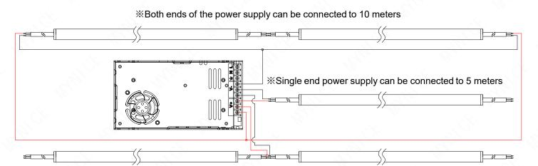
\*The middle power supply, the left and right can be connected to 5 meters a total of 10 meters
