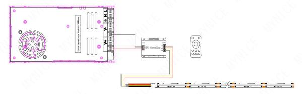
XThe dimmer can be connected to achieve dimming
