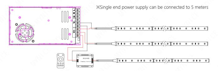
XThe dimmer can be connected to achieve dimming
